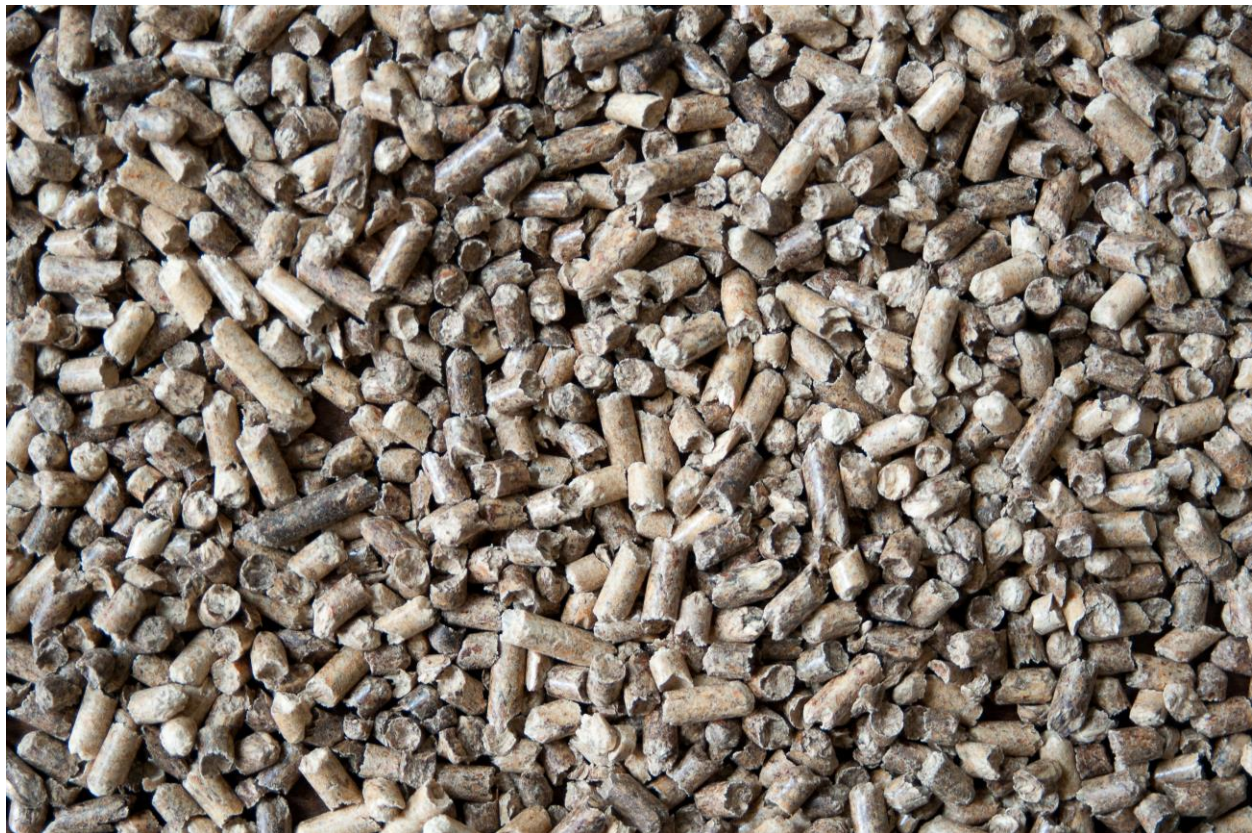
Figure 14. Wood pellets. These pellets were made in British Columbia, Canada, from sawmill residues. Because of current pricing schemes, it is economically feasible to ship them to Europe for use in power stations.
