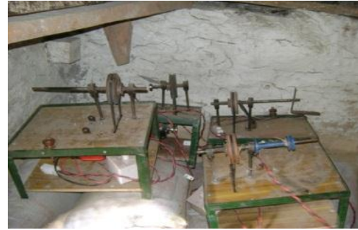
Figure 22 Machinery for lokta paper making
