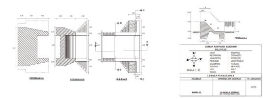
Figure 22. Example of gully control designs
