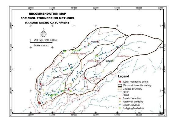
Figure 5. The distributions of points have to be rehabilitated with civil engineering methods in micro catchment scale
